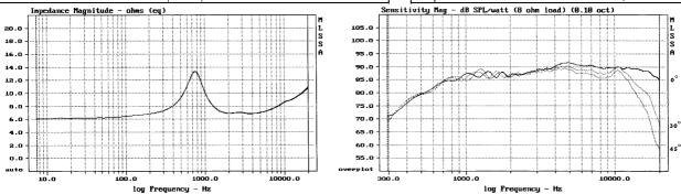
Measured on IEC baffle using Bruel & Kjaer 3144 model microphone. Also available in silver faceplate finish.
